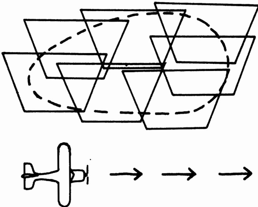
b) correct flight path. No areas are missed and overlap can be worked out.
